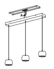
Align the fixture canopy with the mounting plate and secure with the side screws.
